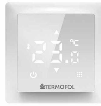
**Specification:** Voltage: 230 V AC 50/60 Hz • color: white | black • internal air temperature sensor: NTC • external air temperature sensor: NTC • maximum switched current: 16A • programmed temperature range: 1÷70 °C • factory programmed temperature range: 5÷35 °C • accuracy: ±0.5 °C • protection level IP31 • external dimensions (without frame): 55 mm x 55 mm • external dimensions (with frame): 82 mm x 82 mm (modular system available)
