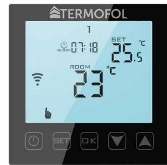
**Specification:** Power consumption < 3 W • voltage: 230 V AC 50/60 Hz • maximum switching current: 20A • range of programmed temperature: 1÷99 °C • factory range of programmed temperature: 5÷35 °C • internal air temperature sensor • accuracy: ±0.5 °C • protection level IP20 • external floor temperature sensor: NTC • control manual • programmable • installation method: surface-mounted • color: white | black • external dimensions: 86 mm x 86 mm x 37 mm
