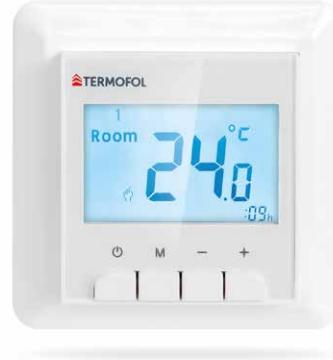
**Specification:** Power consumption < 1.5 W • voltage: 230 V AC 50/60 Hz • maximum output load: 16A • programmable temperature range: 10÷70 °C • limitation of the maximum temperature of the heater - floor: 10 °C - 70 °C • 2 sensors: built-in air temperature sensor + floor temperature sensor - NTC sensor • IP20 protection level • manual control • programming possible • installation method: flush-mounted • color: white • 5+2 temperature programming (5 days a week + weekend)
